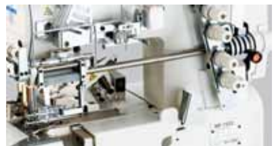
Adjustment of the tape feeding amount
